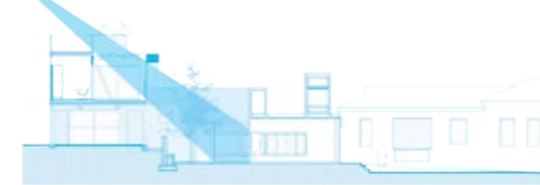
SOLAR ACCESS DIAGRAMS HELP ANTICIPATE THE WAY A SPACE WILL BE NATURALLY ILLUMINATED.
