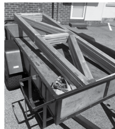
Shutter Prototype Gang-nailed trusses
