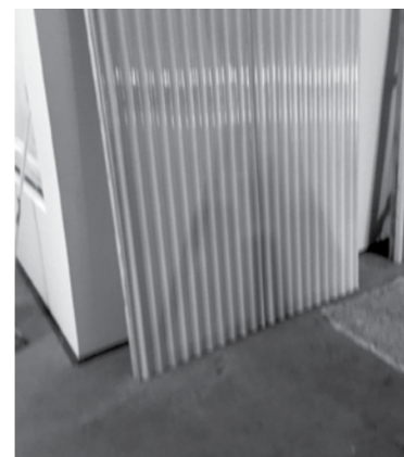
CLADDING: translucent fibre-glass
